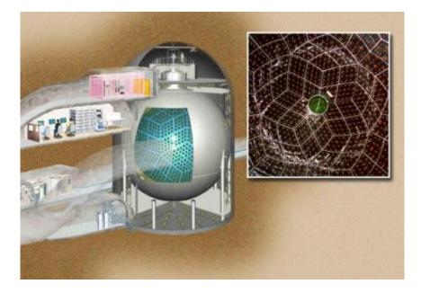
The KamLAND anti-neutrino detector is a vessel filled with scintillating mineral oil and lined with photomultiplier tubes (inset), the largest scintillation detector ever constructed, buried deep underground near Toyama, Japan. Credit: KamLAND Collaboration
