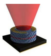
Using an epitaxial approach, University of Illinois researchers developed a 3-D photonic crystal LED, the first such optoelectronic device. Credit: Erik Nelson
