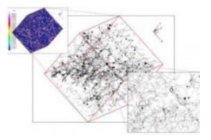
This figure is a presentation of viscous stress and Reynolds stress at multiple micro-spatial scales under ultra-high temperature and pressure conditions. Credit: ©Science China Press
