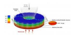
In this diagram of the Sandia Cooler, heat is transferred to the rotating cooling fins. Rotation of the cooling fins eliminates the thermal bottleneck typically associated with a conventional CPU cooler. (Diagram courtesy of Jeff Koplow)
