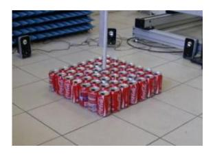
The Coke can acoustic lens, surrounded by speakers, can focus sound waves to a space 1/25th the size of a wavelength. Image credit: Fabrice Lemoult
