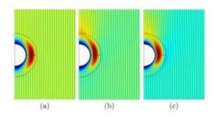
Velocity pro le and streamlines of flow around and through the porous spherical shell surrounded by a viscous fluid. (See ref. below for details). Image credit: arXiv:1106.2282v1
