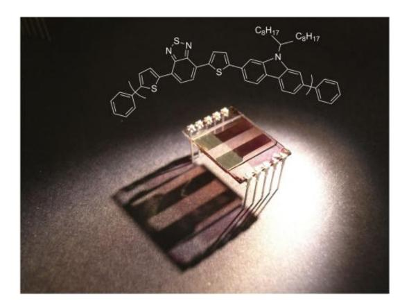
A polymer solar cell ready for testing; the metal connections allow us to measure different areas of the film and measure the device efficiency amongst other parameters. Credit: Andrew Parnell
