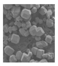
This is a scanning electron microscope image of a new material that self-assembles into a polyhedron using the attractive interactions associated with hydrogen bonds. The shapes then further organize into a crystal lattice that resembles a porous structure called zeolite, an absorbent material with many industrial uses. Credit: Michael D. Ward, New York University
