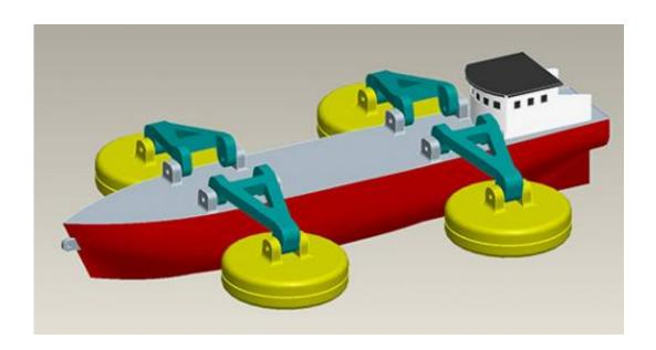
(PhysOrg.com) -- At the Clean Technology 2011 Conference and Expo in Boston, Andre Sharon presented a new concept of using ships equipped with a wave-power system to harvest energy and deliver it back to a power grid on shore.
