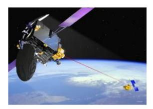
Carrying three payloads plus a number of experiments, Artemis (Advanced Relay and Technology Mission Satellite) has been designed to test and operate new telecommunications techniques. The L-band mobile payload allows two-way
