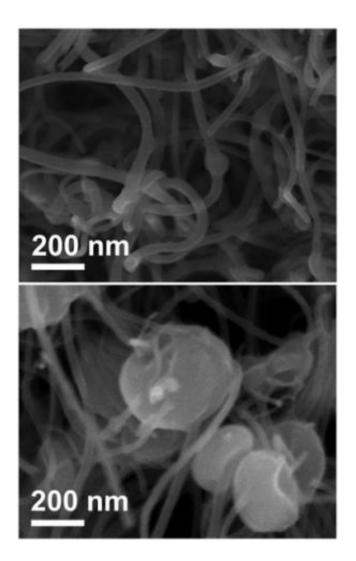
As the battery is used, particles of lithium peroxide form as small dots on the sides of carbon nanofibers (top), and eventually assume larger toroidal (donut) shapes as the battery continues to discharge (bottom), as seen in these scanning electron microscope images. Photo: Courtesy of Mitchell, Gallant, and Shao-Horn
