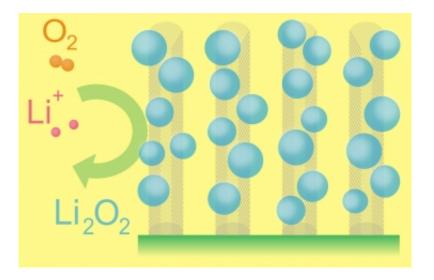
This diagram depicts the essential functioning of the lithium-air battery. Ions of lithium combine with oxygen from the air to form particles of lithium oxides, which attach themselves to carbon fibers on the electrode as the battery is being used. During recharging, the lithium oxides separate again into lithium and oxygen and the process can begin again. Graphic: Courtesy of Mitchell, Gallant, and Shao-Horn
