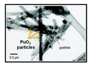
New research demonstrated the effect of goethite on reduction of Pu(IV) by measuring the time dependence of total aqueous Pu concentration, its oxidation state, and system pe/pH.
