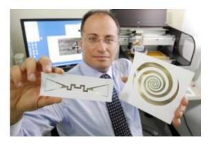
Georgia Tech School of Electrical and Computer Engineering professor Manos Tentzeris holds a sensor (left) and an ultra-broadband spiral antenna for wearable energy-scavenging applications. Both were printed on paper using inkjet technology.
