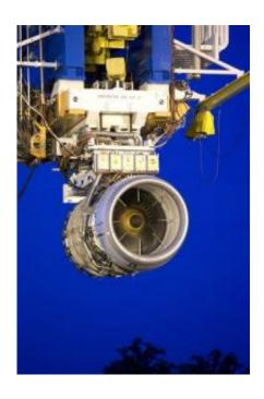
In this undated photo provided by CFM International, the newly designed LEAP turbofan engine is being tested. The lower weight is helping the engine provide a 15% reduction in fuel consumption and well as a 15% reduction in carbon emissions.(AP Photo/CMF International)
