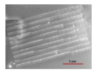
Scanning electron microscope image shows a large PZT line array crystallized on a 240-nanometer thick precursor film on a platinized silicon wafer. Credit: Courtesy of Yaser Bastani
