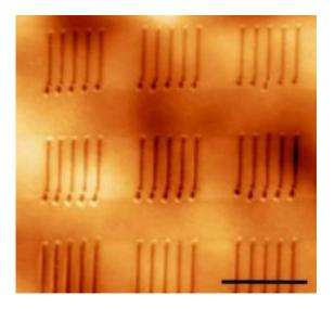
This image shows the topography (by atomic force microscope) of a ferroelectric PTO line array crystallized on a 360-nanometer thick precursor film on polyimide. The scale bar corresponds to one micron. Credit: Courtesy Suenne Kim
