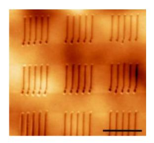
This image shows the topography (by atomic force microscope) of a ferroelectric PTO line array crystallized on a 360-nanometer thick precursor film on polyimide. The scale bar corresponds to one micron. Credit: Courtesy Suenne Kim
