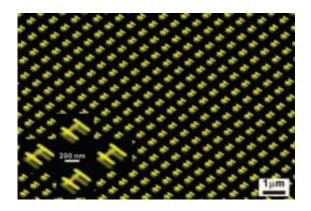
Scanning electron micrograph of 3D plasmon rules fabricated from gold nanorods by electron beam lithography.
