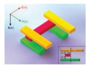
The 3-D plasmon ruler is constructed from five gold nanorods in which one nanorod (red) is placed perpendicular between two pairs of parallel nanorods (yellow and green). Credit: courtesy of Paul Alivisatos research group, Berkeley,
