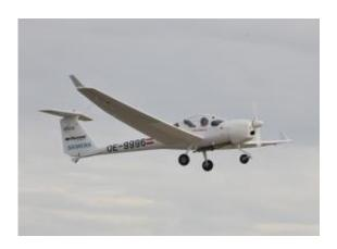
Electromobility is now making inroads into the world of aircraft. The technology of the series hybrid electric drive is scalable and will be used in small and medium-sized aircraft and, in the medium term, larger planes. It will make aviation greener.
