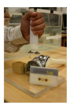
Ortho-Tag would be affixed to an orthopedic implant and scanned via radio-frequency with a probe and RFID tag developed at Pitt. A card (foreground) would be available to patients with an existing implant. Credit: U of Pittsburgh
