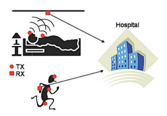
Body-area networks under development at Oregon State University may hold the future of medical monitoring. Data might first be transmitted at a low data rate to a local storage sensor, then received by a doctor at a high data rate. Such approaches may improve medical care, cut costs and help prevent or treat disease. (Graphic courtesy of Oregon State University)
