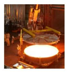
Casting of a 4 meter mirror substrate made of "Zerodur" glass ceramic on June 2, 2006 at SCHOTT headquarters in Mainz, Germany. The molten glass is heated to more than 2,732 degrees Fahrenheit (1,500 degrees Celsius). After cooling and preliminary processing, the substrate is ceramized in an 11-month process in which the glass is transformed to glass ceramic. (Image: SCHOTT)
