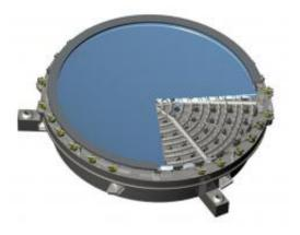
The curved mirror will be manufactured such that it can be adjusted to suit the surrounding conditions using actuators and controlled ventilation on its backside. (Image: AURA)
