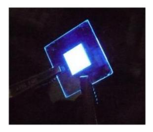
Blue organic light emitting diode (OLED) using new material
