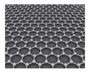
Made of a single sheet of carbon atoms, graphene can be spun at the fastest rate of any known macroscopic object. Image credit: Wikimedia Commons.
