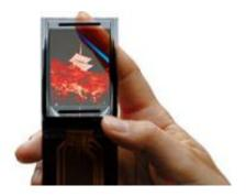
TDK Corporation has started mass production of a newly developed seethrough passive matrix type QVGA organic EL display (product name: UEL476) from this Spring, a world's first.
