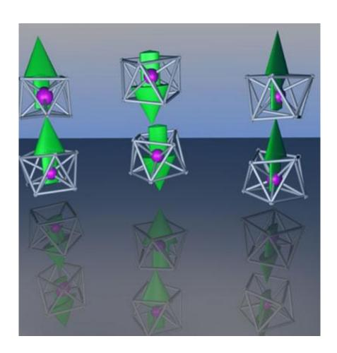
A proposed assembly of FeMg8 magnetic superatoms where the directions of magnetic moment is indicated by arrows. Image courtesy of Victor Medel/VCU.
