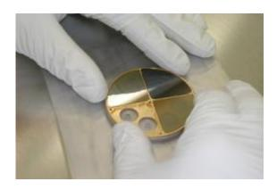
The Solar Wind Concentrator is a special instrument built by a team at Los Alamos National Laboratory to enhance the flow of solar wind onto a small target to make possible oxygen and nitrogen measurements. Shown here, the target section of the concentrator, which produced essential samples of nitrogen and oxygen.
