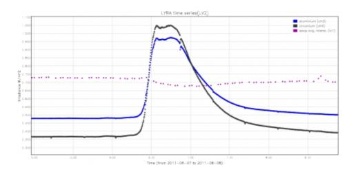
Proba-2's LYRA (Large Yield Radiometer) instrument measures the energy intensity of the Sun across four separate ultraviolet bands every 50 milliseconds, observing a spike in signal across its two short-wavelength bands due to the 7 June 2011 solar flare. The flare caused a decrease in the SWAP average intensity from Proba-2's other Sun-watching instrument, shown in here purple. Credits: ROB
