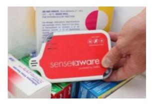
The sensor can keep tabs of where a package is located, if it has been opened, and more. Credit: Strouse/NIST
