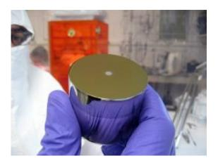
Juan Collar, associate professor in physics, holds one of the early germanium detector prototypes similar to the one being used in the Coherent Germanium Neutrino Technology (CoGeNT) experiment, situated nearly half a mile deep in the Soudan Mine in Minnesota. Such underground locations help screen out false dark-matter signals from other natural sources of radiation. Detectors of this kind are used because of their sensitivity to weak levels of radiation. Courtesy of CoGeNT Collaboration
