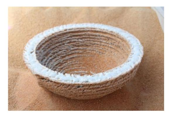
This new 3D model gets is based on current designs of 3D <u>printing</u> <u>technology</u> with only two substitutions. The traditionally used resin or plastic powder has been replaced by the sand and the laser has been
