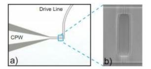
a) Optical micrograph of the device. Light parts are Al while dark parts are the Si substrate. The output line is labeled "CPW" and the drive line enters from the top. Both lines converge near the SQUID. b) A scanning-electron micrograph of the SQUID. Image credit: arXiv:1105.4714v1
