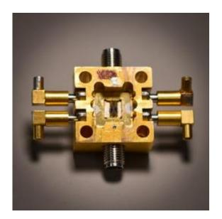
A superconducting circuit (small square, center) fits snugly into a housing that enables it to receive electrical signals inside a cooling tank. Credit: Melanie Gonick
