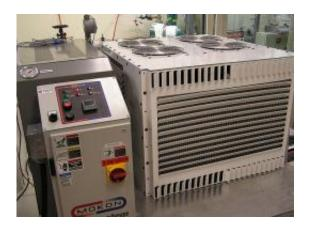
This prototype of a "thermal activated cooling system" has been developed by engineers at Oregon State University, and promises important new advances in energy efficiency by using wasted heat. (Photo courtesy of Oregon State University)
