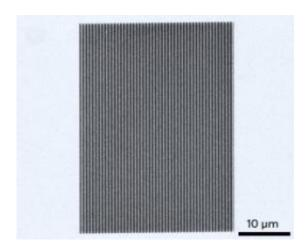
A scanning electron microscope image of an organic grating used to excite surface plasmons.
