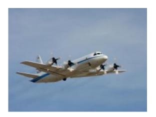
NASA's P-3B is a four-engine turboprop, capable of long duration flights of 8 to 12 hours and is based out of NASA's Wallops Flight Facility in Wallops Island, VA. Credit: NASA
