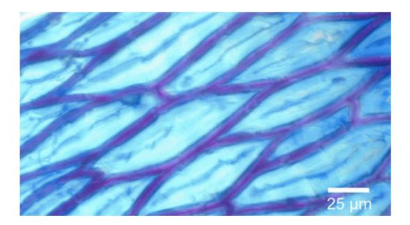
The honeycomb structure that has become saturated with water and preferably expands in one direction. The researchers have stained the swellable cellulose blue. The lignin in the cell walls is stained red. © Matt Harrington/ MPI of Colloids and Interfaces
