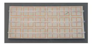
NIST's fluid-tunable "metasurface" consists of copper structures and plastic tubing mounted on composite board. The presence of water in the tubing changes the resonant frequency at which the metasurface absorbs and stores energy. Credit: NIST
