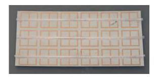
NIST's fluid-tunable "metasurface" consists of copper structures and plastic tubing mounted on composite board. The presence of water in the tubing changes the resonant frequency at which the metasurface absorbs and stores energy. Credit: NIST
