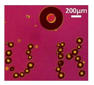
A photomicrograph showing the microrobot built by the University of Hawaii (circular object in top center) along with a series of glass beads that it assembled into a mini "U H". The 200 micrometer scale bar in the upper right corner is about the length of a parametium. Credit: Ohta/University of Hawaii at Manoa
