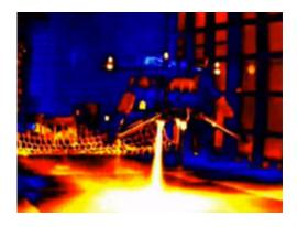
Infrared image of hover test of the robotic lander. (NASA/MSFC)
