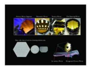
This image shows the four different types of mirrors on the Webb telescope. From left to right are: a primary mirror segment, the secondary mirror, tertiary mirror and the fine steering mirror. The bottom right shows an artist's conception of the Webb telescope optics with its 18 primary mirror segments. Credit: NASA/Ball Aerospace/Tinsley
