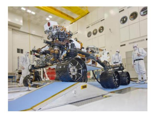
This photograph of the NASA Mars Science Laboratory rover, Curiosity, with its left-front wheel on a ramp was taken during mobility testing on June 3, 2011. The location is inside the Spacecraft Assembly Facility at NASA's Jet Propulsion Laboratory, Pasadena, Calif. Credit: NASA/JPL-Caltech
