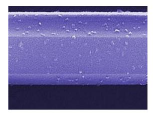
Scanning electron microscope image of a gas sensor segment fabricated of a semiconducting nanowire of gallium nitride. The nanowire of less than 500 nanometers across is coated with nanoclusters of titanium dioxide, which alters the current in the nanowire in the presence of a volatile organic compound and ultraviolet light. Credit: NIST
