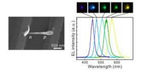
(Left) A single nanodisk-nanorod LED viewed with a field-emission scanning electron microscope. (Right) Some colors of light emissions from nanodisk-nanorod LEDs - violet, blue, cyan, green, and yellow - viewed with an optical microscope. Image credit: Lu, et al. ©2011 American Institute of Physics
