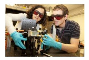
Serpil Kucuker Dogan and Matthew Musgrave work on a helium-3 cell that is used to measure the angle at which the neutron beam strikes the liquid hydrogen sample.
