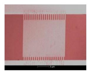
Colorized micrograph of an ultrafast single-photon detector made of superconducting nanowires. NIST researchers use electron beam lithography to pattern the nanowires (vertical lines) on a thin film of tungsten-silicon alloy, which produces more reliable signals than the niobium nitride material used previously. Credit: Credit: Baek/NIST
