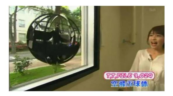
(PhysOrg.com) -- Researchers working with the Japanese Ministry of Self-Defense have created what they claim is the worlds first completely spherical flying robot. The robot, which has roughly the same dimensions as a soccer ball, is able to travel at speeds of up to 40 miles per hour, or hover in the general area of a stable spot such as a hallway.
