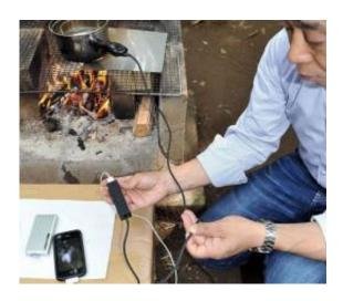
A member of Japanese electronics venture TES NewEnergy unveils a pot that can charge mobile phones while boiling water for use in earthquake and other emergency situations, at a demonstration in Tsukuba City in Ibaraki prefecture on June 9. The Hatsuden-Nabe thermo-electric cookpot turns heat from boiling water into electricity that feeds via a USB port into digital devices such as smartphones.
