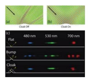
When an input beam (black arrow) reflects off (a) a bump without a cloak, the bump causes a perturbation. When the beam reflects off (b) a bump covered by a cloak, the cloak masks the bump, and the reflected beam is reconstructed as if the bump did not exist. (c) Light after reflection from a flat mirror, a bump without a cloak, and a cloaked bump, at three different wavelengths. Image credit: Majid Gharghi, et al. ©2011 American Chemical Society
