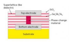
A schematic illustration of a phase-change memory element incorporating a superlattice-like dielectric.
