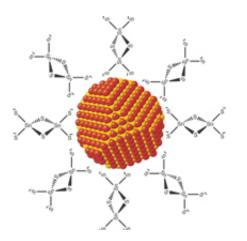
Inorganic surface ligands enable facile electron transport between quantum dots and opened novel opportunities for using nanostructures in solar cells.
