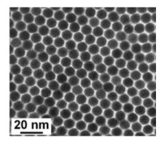
Arrays of quantum dots allow fabrication of solar cells by printing and other inexpensive techniques.
