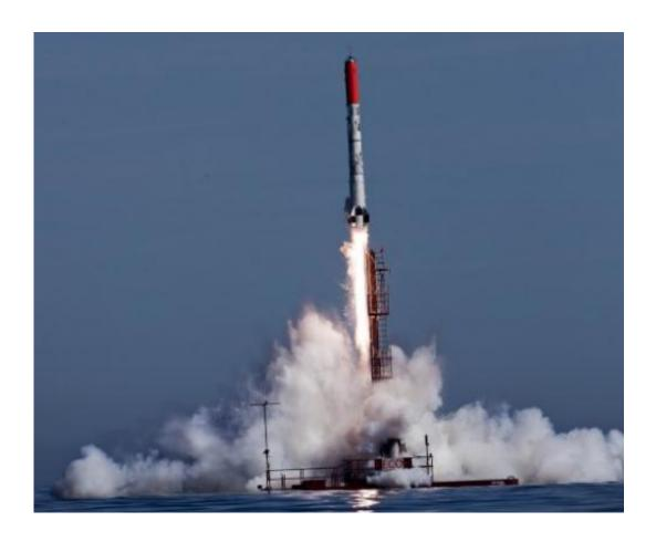
Danish amateur rocket, Heat-1X Tycho Brahe, a MSC (micro spacecraft), launches in the Baltic Sea east of Bornholm, carrying a doll of human size. The goal for the Danish amateur rocket builders was to send the rocket 15 to 16 Km up in the air, but it reached only 2,8 km and flew a total of 8.5 km.
